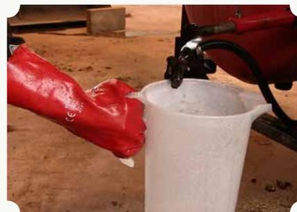
Next we need to measure the water output of the nozzles. Once the sprayer is set up with the right nozzles and the pressure is selected, run the spray with clean water in the tank and measure the output of each individual nozzle for 1 minute. Measuring each nozzle will indicate if any of them are out by more than 10%, if so they should be replaced. Add the measurement for all nozzles together to get you total output per minute in litres.
