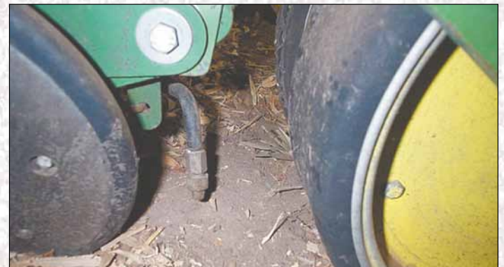
Spray nozzle set up to apply Rizolex InFurrow in the furrow after seed and fertiliser placement.
