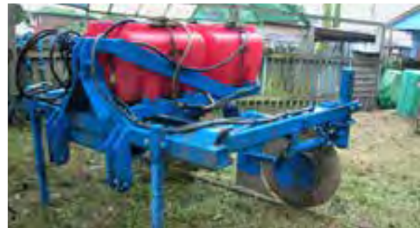
FIGURE 7: A two row hydraulically adjustable coulters applicator with a second mixing tank and nozzles set up to apply herbicide to the base of tree rows at the same time as Shield Systemic Insecticide is applied sub-surface. This machinery is patented. Contact your Sumitomo Chemical representative for more information.
