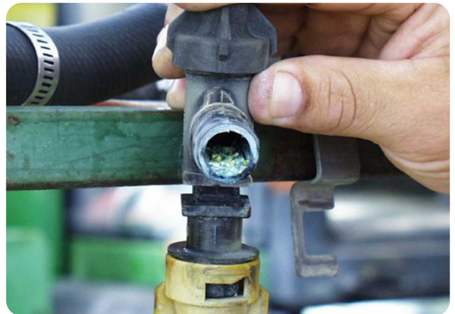
Inside diaphragms. This problem is particularly common for air-assisted sprayers.
